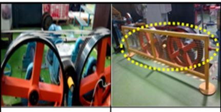
farlier :- There were no cover. Chances of rire hitting the operator during wire breakage
