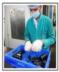
For parts like KVNF deflashing is now done at molding stage only resulting in increase of productivity, removal of defalshing operation and also reduce rejection percentage from 5% to 3.3%
